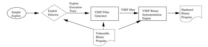
Figure 1. VSEF architecture. Once an exploit is detected, an execution log is produced. The VSEF Filter Generator produces a filter that recognizes execution patterns that exploit the vulnerability. These filters can then be disseminated. The VSEF Filter Generator takes the filter and instruments the binary to recognize execution sequences that exploit the vulnerability, the result being a hardened binary.
