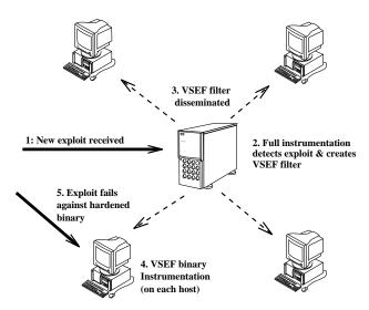
Figure 2. The deployment scenario for vulnerability-specific execution filtering. Upon (1) receiving an exploit of a new vulnerability, the (2) full instrumentation engine detects it and creates an appropriate filter. The filter is (3) disseminated to all hosts, which then (4) use the filter to instrument and produce a hardened binary. The hardened binary cannot be then exploited (5). Note that the exploit in step 5 may be a polymorphic variant of step 1.
