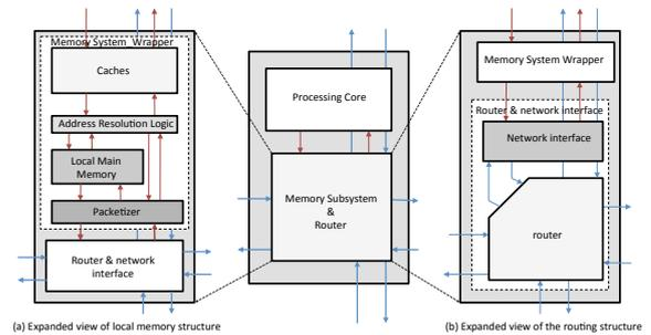
Fig. 2. Network node structure.
