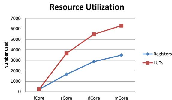
Fig. 3. FPGA resource utilization per core.
