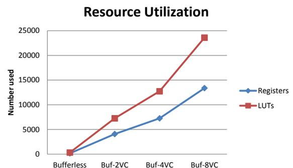
Fig. 6. FPGA resource utilization per router configuration.
