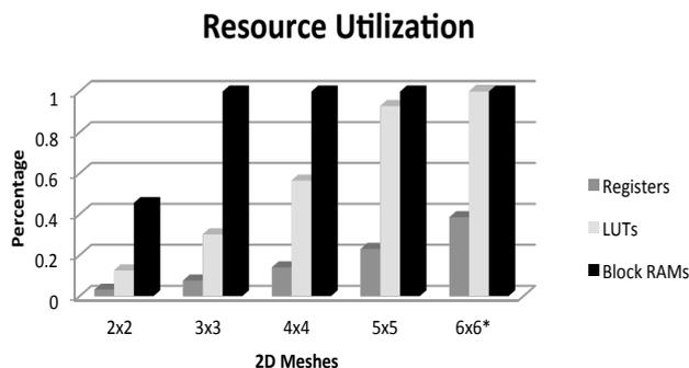
Fig. 10. Percentage of FPGA resource utilization per mesh size.
