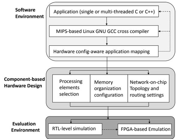
Fig. 1. *Heracles*-based design flow.
