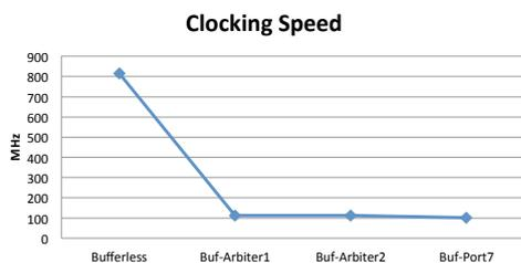
Fig. 8. Clocking speed of different router types.
