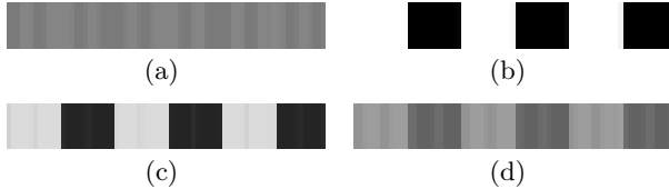
Figure 3: Images as seen by a camera of a surface illuminated by an LED pulsing at (a) 1kHz (b) 100kHz. Mixed low-speed and high-speed communication with (c) 15-85% duty cycle (d) 40-60% duty cycle
