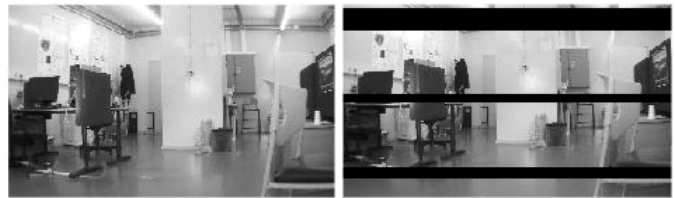
Fig. 16. Snapshot of the video stream at the sink. With CSMA/CA (on the right), relays cannot handle every received packet, dropping some that appear as black lines in the image. Under DVSP (on the left), video streaming is visibly improved and frames are generally complete.
