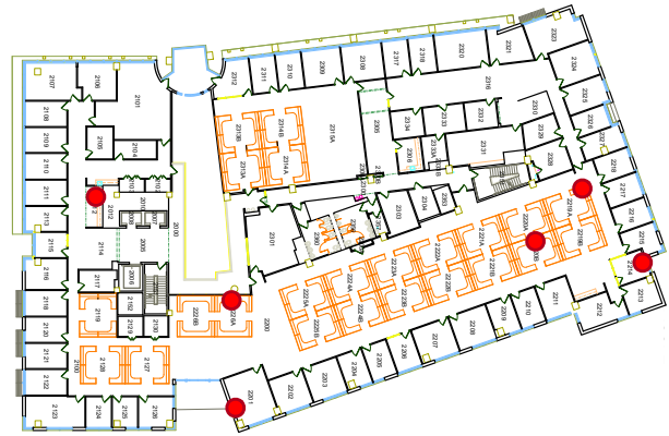
Figure 8: Experimental LoRaWAN test-bed layout: there are 6 gateways in total, spread across an indoor office environment. Each red dot indicates a LoRaWAN receiver.
