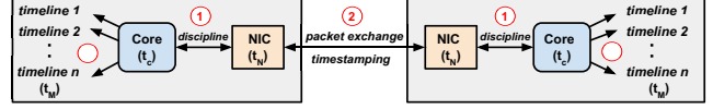
Fig. 5: End-to-end time synchronization using timelines. (1) NIC is disciplined by the core clock on a single node ( t_N = t_C ). (2) NICs on two nodes exchange packets and timestamp them in core time. (3) The timestamps are used to work out the Core – Core mapping ( t_M ) and are stored in the form of a logical timeline mapping.
