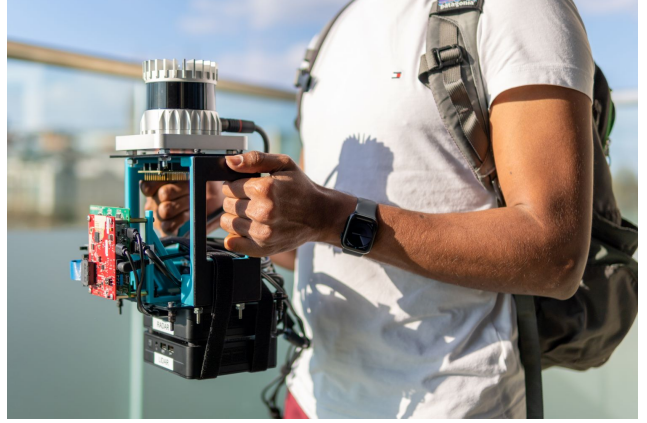
Figure 15. Our data collection system consists of a handheld rig (Fig. 6) and a backpack which carries power equipment.
