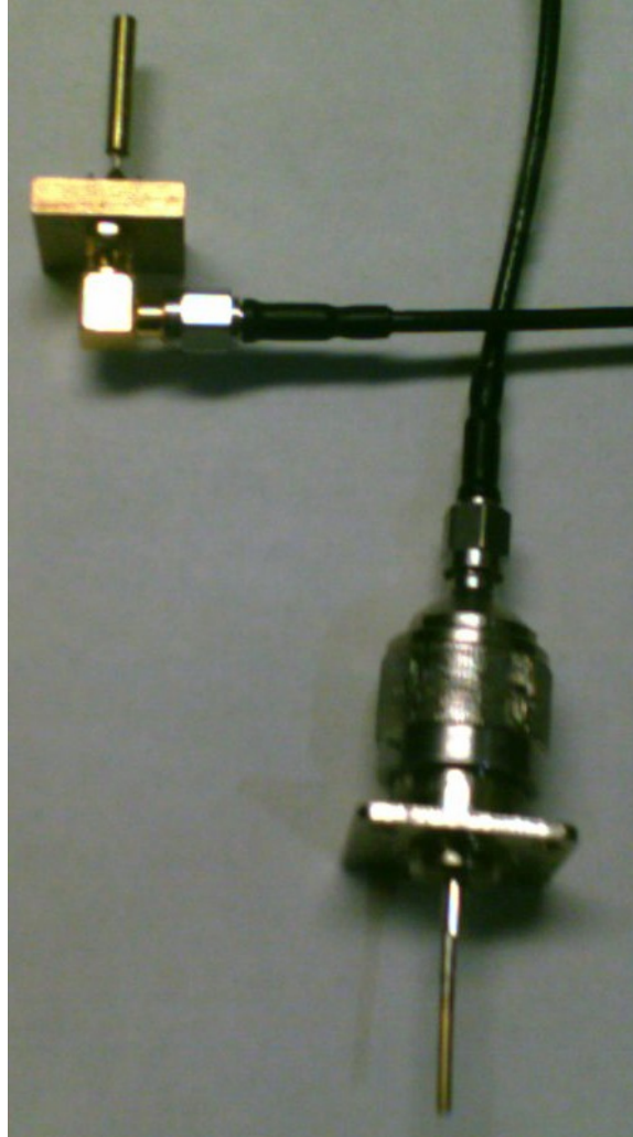
Figure 2.13: A more complicated duct re-radiator system. The upper antenna is inserted into the ventilation duct while the lower antenna is mounted between two metal KlimaTak acoustical panels in the ceiling and a short run of coaxial cable is run between the two.
