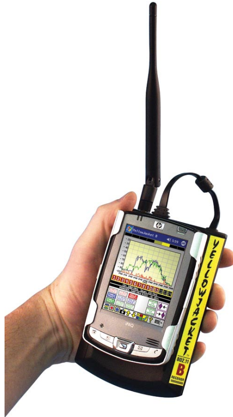
Figure 2.15: A Berkeley Varitronics' YellowJacket IEEE 802.11b scanning receiver of the type used for measuring received signal strength in the re-radiator comparison measurements. Picture excerpted from [30].
