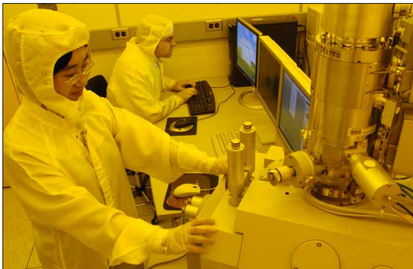
Newly installed FEI Sirion 600 scanning electron microscope and Nabyty NPGS electron beam lithography system with 10 nm writing resolution of complex shapes on up to six-inch diameter wafers. PhD students Matthew Moneck and Chun Wang pictured training to use the system. (Photos Courtesy of Ken Andreyo of CMU)
