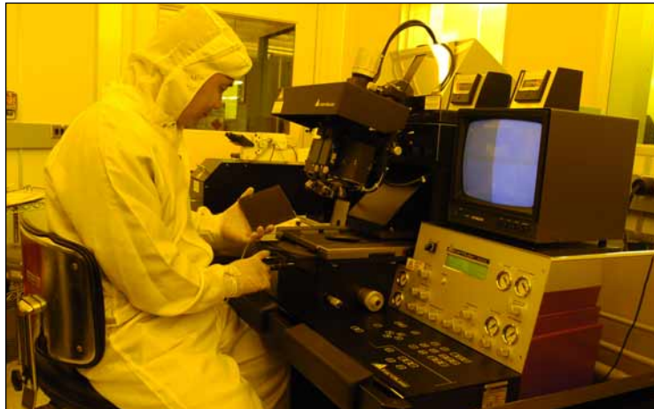
Karl Suss MA6 backside wafer/bond aligner with near field holography system and fixturing for small chips to six-inch diameter wafers. Han Dong of Bridge Semiconductor pictured preparing to load a mask.
