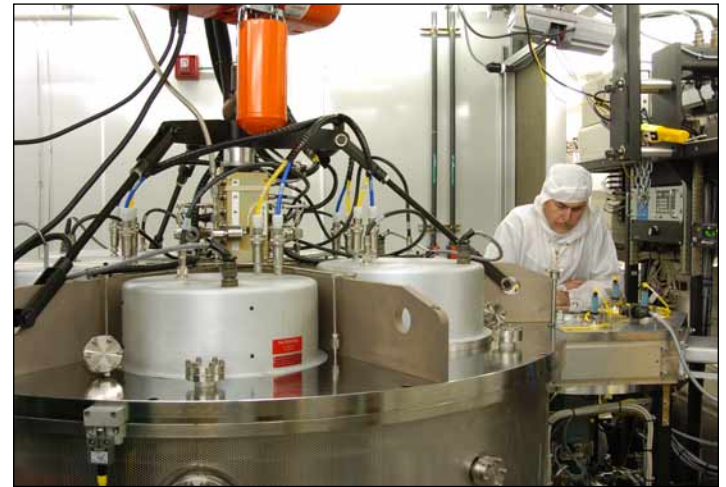
CVC Connexion sputtering system process chamber each with six each twelve-inch diameter sputtering cathodes. Chris Bowman pictured looking into the wafer exchange chamber.
