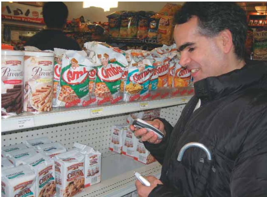
Figure 1. Trinetra system. The combination of a barcode-scanning pencil and a smart cell phone lets a blind user distinguish between various grocery products without assistance from a sighted individual.
