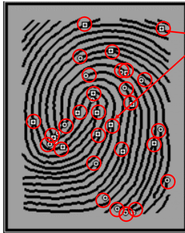
Final Processed with Fingerprint Minutiae Detected
