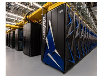
Summit 187.7 Pflop/s, 13 MW 9,216 x 22 cores POWER9 + 27,648 V100 GPUs
