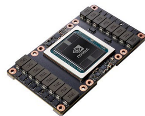
Nvidia Tesla A100 9.7/19.5 Tflop/s, 400 W 6912 cores, 1.4 GHz 32-way SIMT, tensor cores
