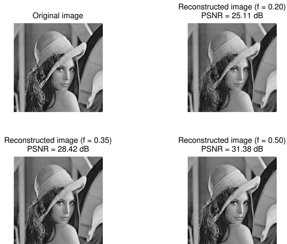
Figure 4.8: Final recovered lena image for different values of undersampling f . The PSNR value is defined as 20 \log_{10} \left( \frac{\max(I)}{\sqrt{\sum_{i=1}^N (I_i - J_i)^2 / N}} \right) , where I and J are the vectorized original and reconstructed images respectively and N is the number of pixels.
