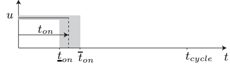
Figure 4: Range of times [\underline{t}_{on}, \overline{t}_{on}] for which the charge pump is switched off. The mode both_active is not considered in this figure.
