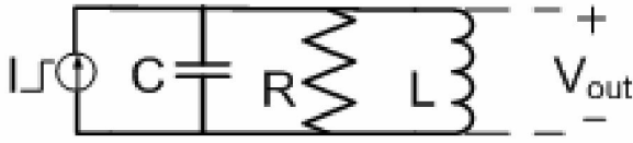
Fig.4. Simplified small-signal power grid network model
