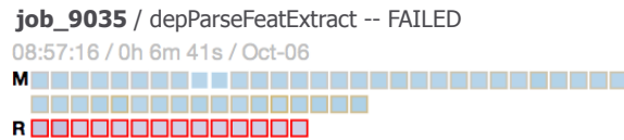
Figure 7: Visual signature of bugs in the Map phase . Failures spread across all Map nodes (solid red border) typically signals a bug in the Map phase.
