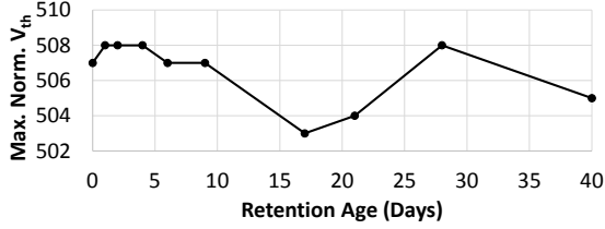
Fig. 8. Maximum threshold voltage within a block with 8K P/E cycles of wear vs. retention age, at room temperature.
