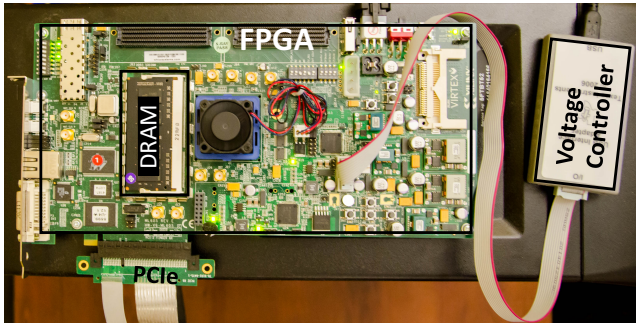
Figure 3: FPGA-based DRAM testing platform.
