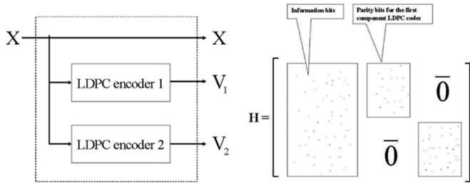
Fig. 1. Left: The encoder structure for the concatenated LDPC codes in [22]. Right: The parity-check matrix  $\mathbf{H}$  for the concatenated LDPC codes in [21], [22].
