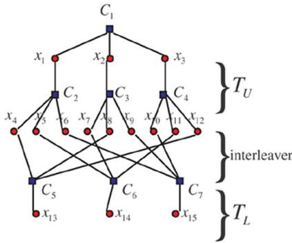
Fig. 21. An equivalent representation of the Tanner graph shown in Fig. 20. (The root of  $T_L$  is removed.)
