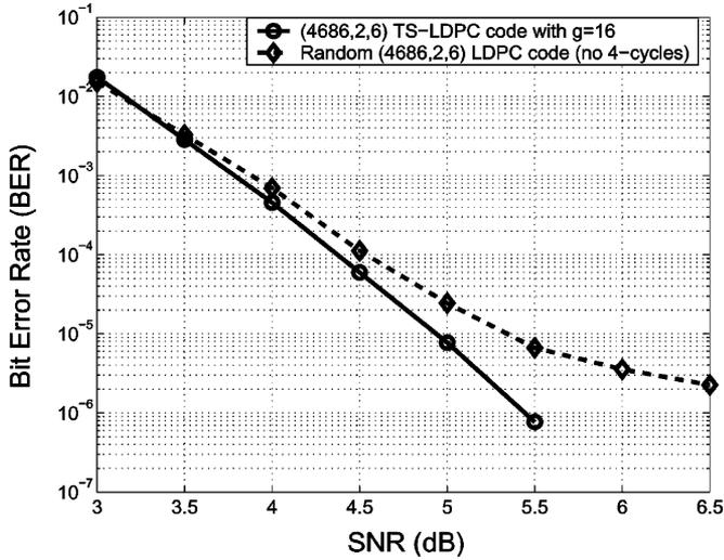
Fig. 14. Comparison of BER performance for a (4686, 2, 6) TS-LDPC code with girth 16, rate 2/3, and a randomly constructed (4686, 2, 6) LDPC code (no 4-cycles).
