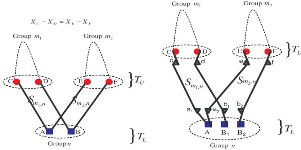
Fig. 9. Left: A type II cycle that can **NOT** be excluded by any choice of the shifts  $S_{m_1,n}$  and  $S_{m_2,n}$ . Right: A subsidiary figure with auxiliary nodes to prove that the cycle shown on the left always exists.
