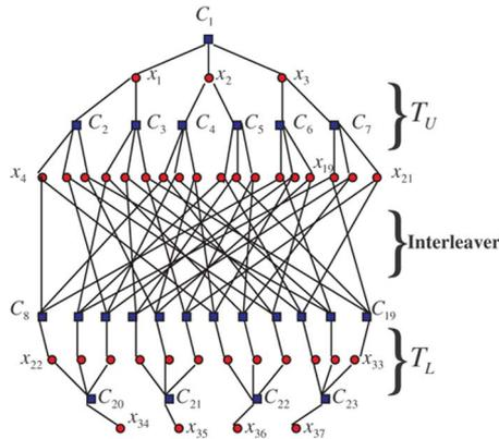
Fig. 23. An equivalent representation of the Tanner graph shown in Fig. 22. (The root of  $T_L$  is removed.)
