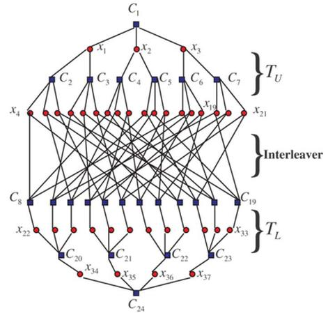
Fig. 22. Tanner graph for an EFTS-LDPC code. (The bit node degree of  $T_U$  is odd.)
