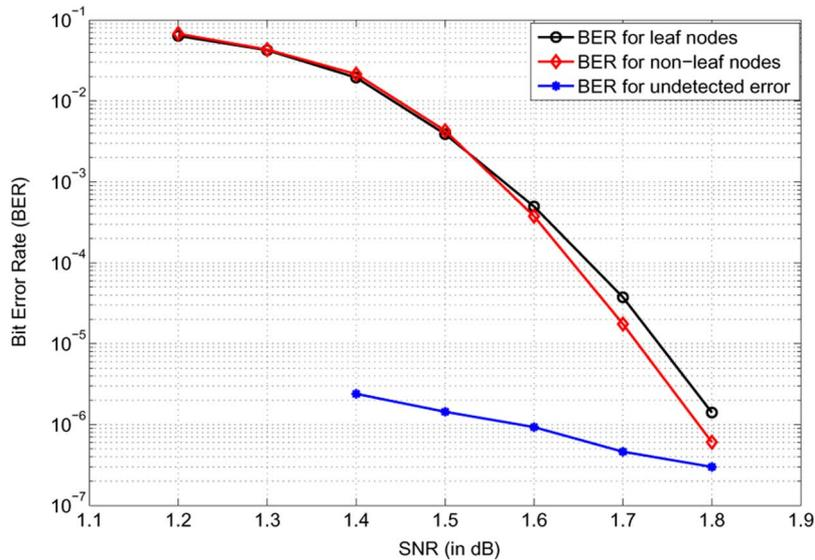
Fig. 18. BER performance of leaf-nodes, nonleaf-nodes, and undetected error events for a (6666,3,6) TS-LDPC code.
