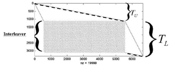
Fig. 3. Parity-check matrix  $\mathbf{H}$  of a (6666, 3, 6) TS-LDPC code with girth 10.
