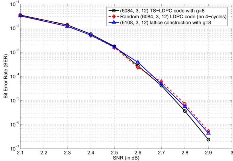
Fig. 15. BER performance comparison between a (6084, 3, 12) TS-LDPC code with girth 8, rate 3/4, a randomly constructed (6084, 3, 12) LDPC code (no 4-cycles), and a (6108, 3, 12) LDPC code on rectangular integer lattices.
