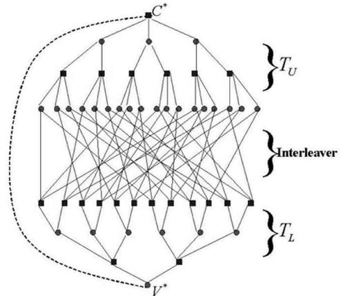
Fig. 2. The decoder Tanner graph of a TS-LDPC code:  $h = 4$ ,  $j = 3$ , and  $k = 4$ .
