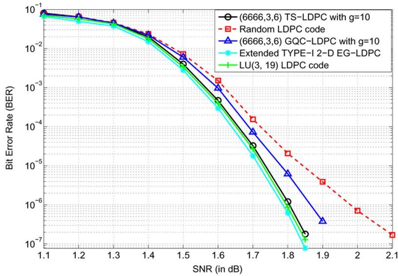
Fig. 17. BER performance comparison between a (6666, 3, 6) TS-LDPC code with girth 10, rate 1/2, a randomly constructed (6666, 3, 6) LDPC code (no 4-cycles), a (6666, 3, 6) GQC-LDPC code with girth 10, rate 1/2, an extended type-1 2-D EG-LDPC code with code block length 8190 and code rate 0.5 (LDPC code based on finite geometries), and LU(3, 19) LDPC code with code block length 6859 and code rate 0.4514.
