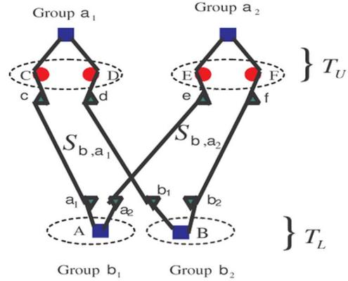
Fig. 12. Divide check nodes  $A$  and  $B$  into subgroups to avoid a length 8 cycle.
