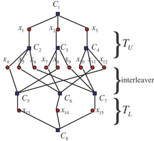
Fig. 20. Tanner graph for an EFTS-LDPC code (The bit node degree of  $T_U$  is even).
