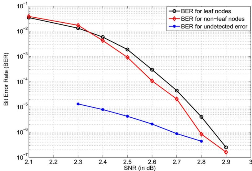
Fig. 16. BER performance of leaf nodes, non-leaf nodes, and undetected error events for a (6084, 3, 12) TS-LDPC code.
