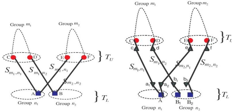
Fig. 11. Left: A type II cycle that **CAN** be excluded by choosing appropriate shifts  $S_{m_1, n_1}$ ,  $S_{m_1, n_2}$ ,  $S_{m_2, n_1}$ , and  $S_{m_2, n_2}$ . Right: An auxiliary figure to show that the cycle shown on the left **CAN** be excluded.
