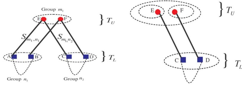
Fig. 13. Left: A type of cycle that can *NOT* be excluded by choices of shifts  $S_{m_1, n_1}$  and  $S_{m_1, n_2}$ . Right: Divide bit nodes  $E$  and  $F$  into subgroups to avoid cycles.
