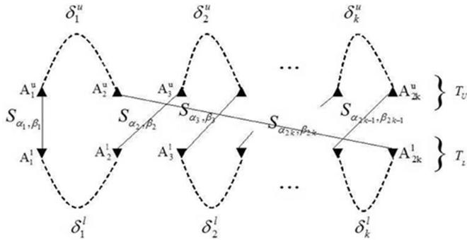
Fig. 8. Type II cycle with  $2k$  edges in the interleaver.
