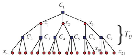
Fig. 24. Upper tree  $T_U$  of an EFTS-LDPC code.
