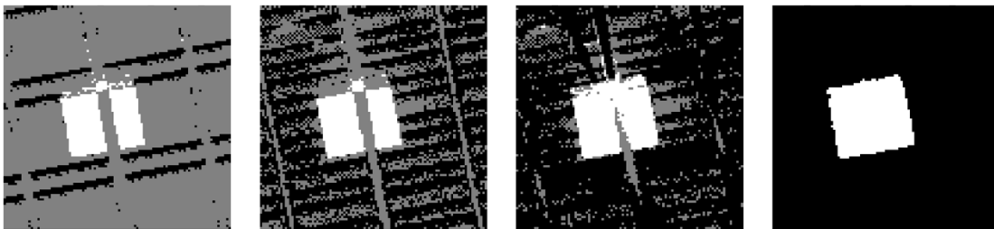
Fig. 14. Estimate of the robot template after frames 2, 4, 6, and 10 of the video sequence of Fig. 13.
