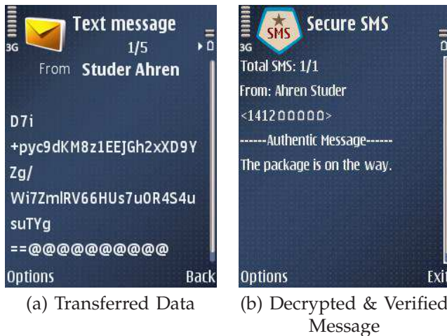
Fig. 7. The data transferred as part of secure SMS and the decrypted message at the receiver.
