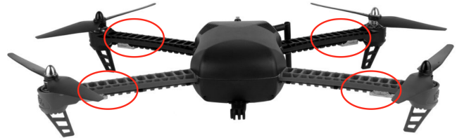
Fig. 1. Quadcopter equipped with microphones (positioned in the red circles) close to each rotor. After classifying the sound of each rotor separately, we fuse the classifier outputs to obtain improved ascend/hover/descend state predictions.
