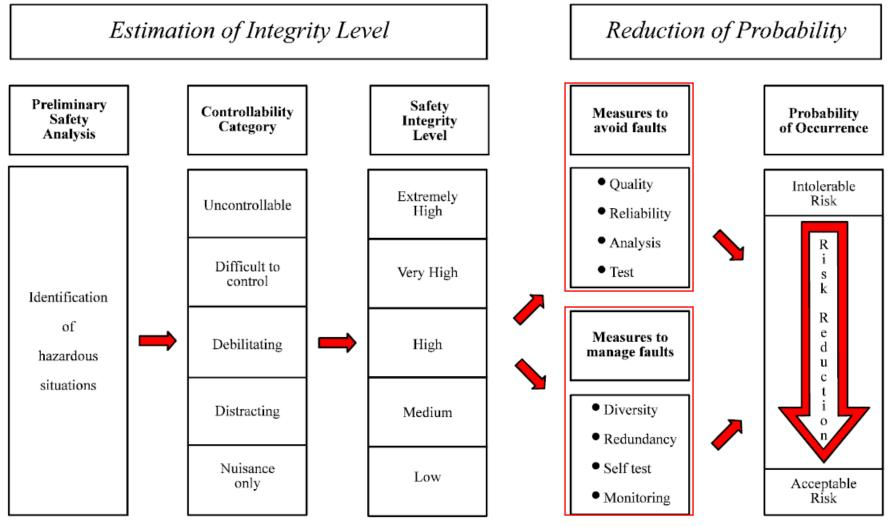
Figure 4 - Approach to avoid hazardous malfunctions
