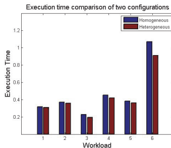
Fig. 3: Execution time for homogeneous vs. heterogeneous configurations
