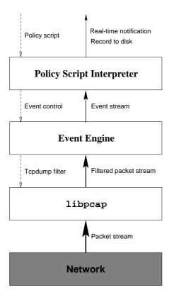
Figure 1: Structure of the Bro system
